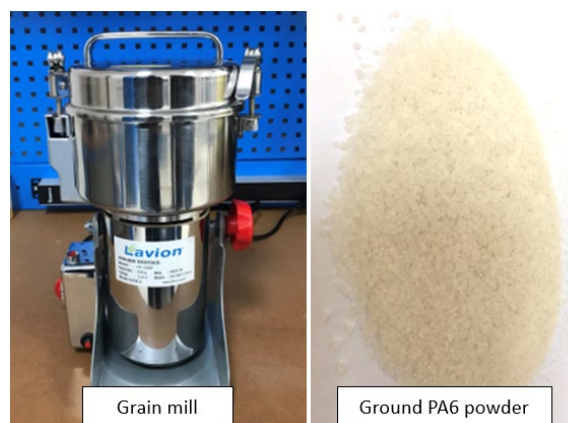
Figure 2. Lavion HC500 Y brand grain mill was used to pulverize and convert PA6 into powder for
