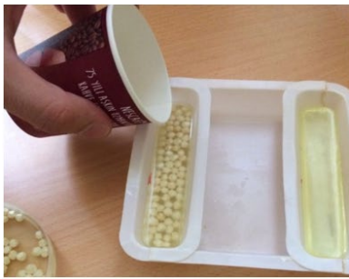
Figure 6. Production of Charpy impact test specimens
