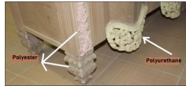
Resim/Figure A: MDF levhadan imal edilen konsol / Console made of MDF board
