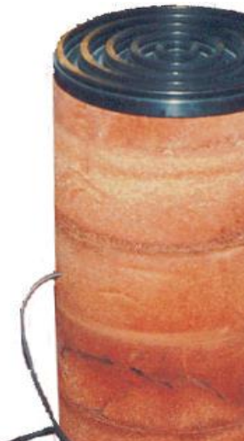
Figure 1. Earth-Air Thermoelectric Generator (EATEG) (Termoelektrik Toprak-Hava Jeneratörü (THTEJ))
