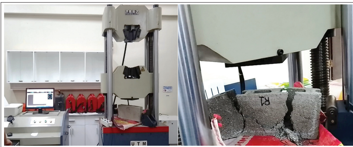
Figure 3. Compressive Testing of the Hollow Concrete Blocks through the UTM .
