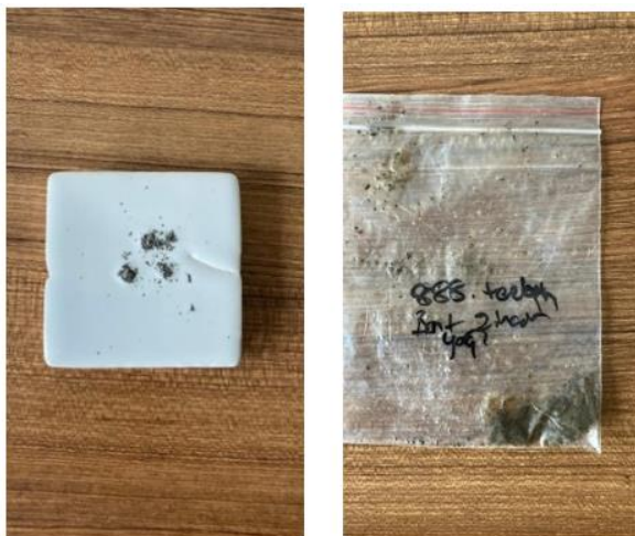
Figure 5. Die casting machine slag materials (Right) and defects caused by them (Left).
