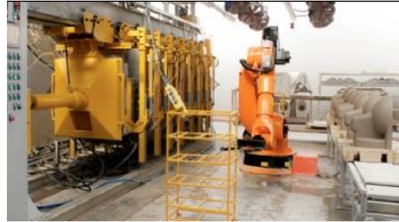
Figure 6. Vitrified die casting machine from Ece Banyo.
