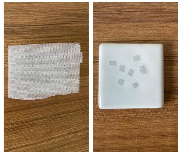
Figure 7. Strip tape abrasive (Left) and defects (Right) due to this abrasion.
