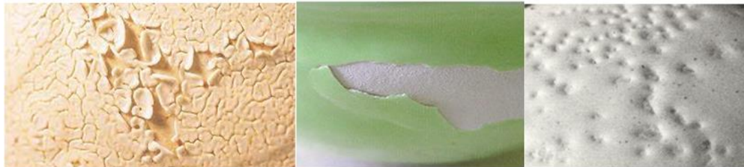
Figure 3. Some ceramic glaze defects ( Hopper, 2023).
