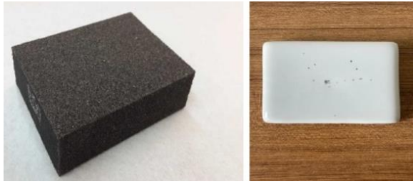
Figure 8. Box Abrasive (Left) and Related Defects (Right).
