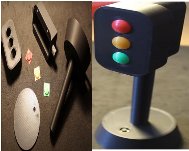
Figure 6. Three-dimensional Printing and Combination of the Traffic Light
