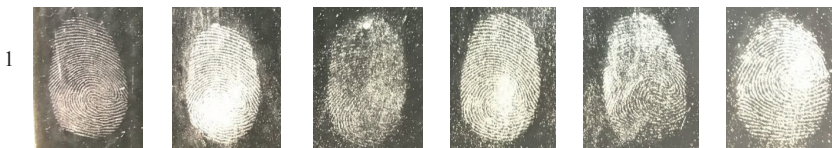
Figure S2. Sebaceous (1) and dry (2) fingerprints developed on rubber surface, using following powder samples: a) BVDA Magnetic silver powder; b) Pure dextran powder; c) S(1/0/0); d) S(1/1/0); e) S(1/0/1) and f) S(1/1/1); and recorded under visible light.
