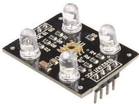
Figure 2. TCS3200 color sensor used to determine the rainbow trout's meat color
