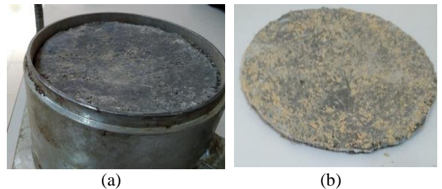
Figure 7. The photographs of cement-coated geotextiles after the experiments a) sand soil b) base material
