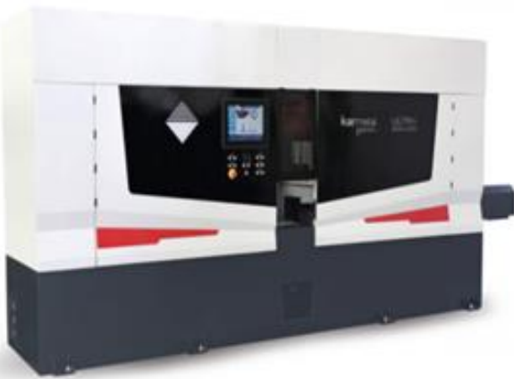
Figure 1. ULTRA 300x300 Fully automatic domestic band saw machine (Production of Kar Metal Company in Turkey)
