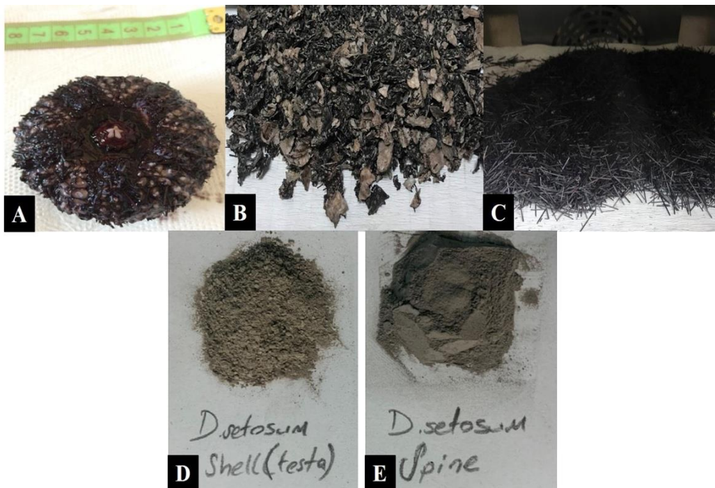
Figure 2. Trimmed and separated form of spines of sea urchins (a) shells (b) and spines (c) divided into two with a pair of scissors of sea urchin, washed with tap water and then with bidistilled water and dried in an oven at 70 °C for 24 hours of the shell (d) and spines (e)
