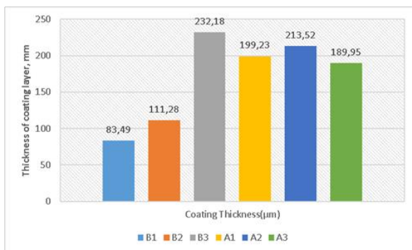
Figure 2. The coating thickness of coated sample by HVOF
