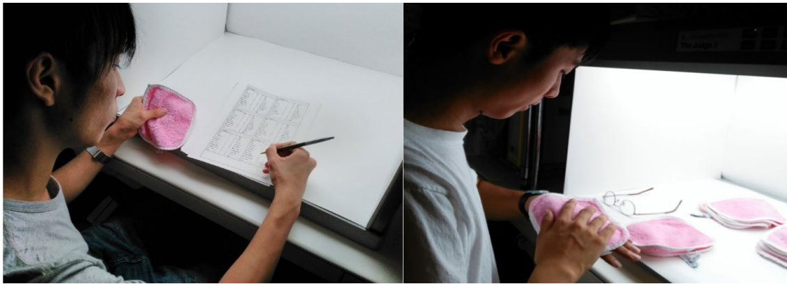
Figure 1. Subjective evaluation is performed in the light cabin under D65 daylight
