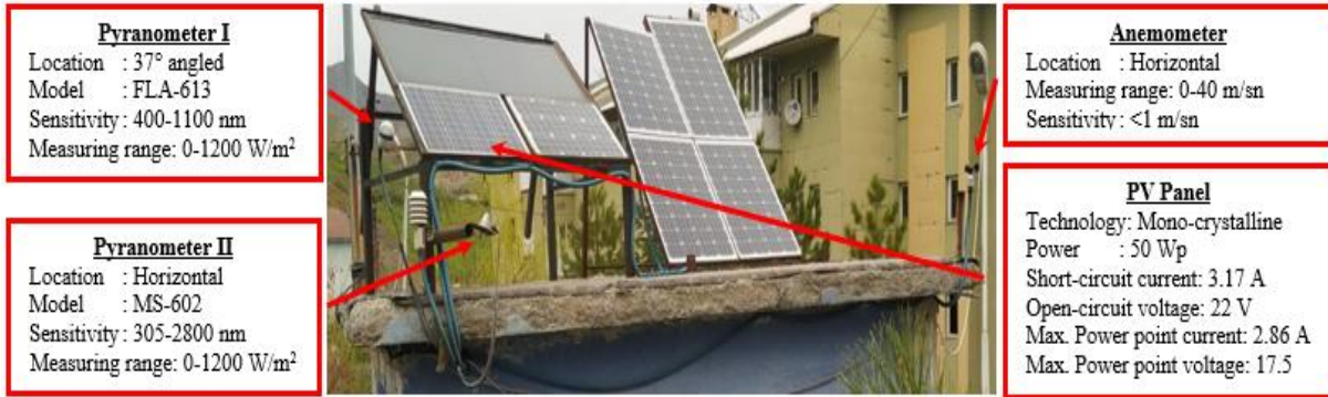
Figure 2. Experimental setup and measurement equipment of Hakkari University meteorological station.
