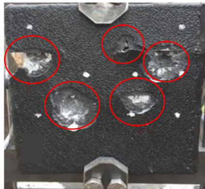
Figure 25: Standalone Ceramic Composite Armor System View after Ballistic Test.
