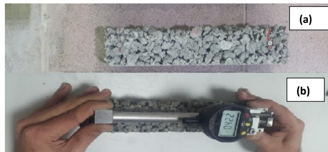
Figure 1: (a) Sample with two demec points; (b) Dial gauge machine.
