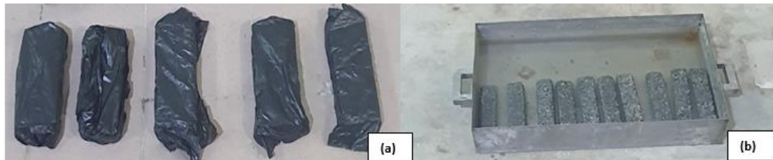
Figure 2: (a) Specimens of autogenous shrinkage; (b) Specimens of expansion.
