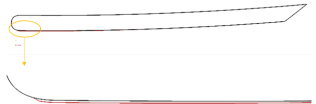
Figure 22. Initial (Black) and Optimized (Red) Vane Blade Profiles
