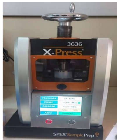
Figure 2. Press machine with 30 tons capacity.
