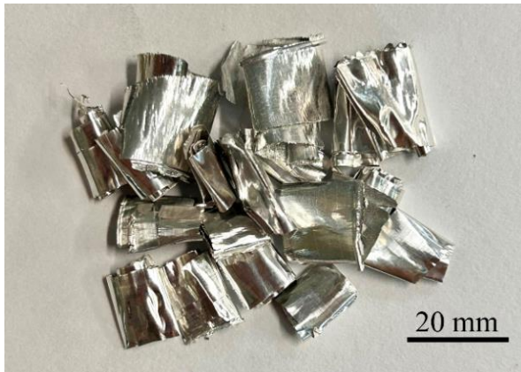
Figure 1. AZ63 chips used for the remelting experiments.
