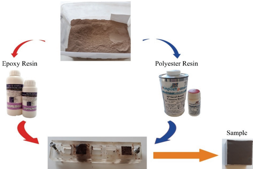
Figure 1 - Production stage of composite mortars.
