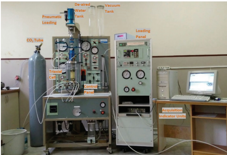
Figure 2 - Dynamic triaxial testing system
