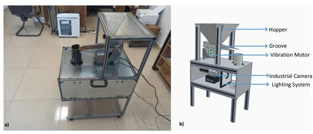
Figure 1. (a) Experimental setup (b) Working principle of experimental setup.
