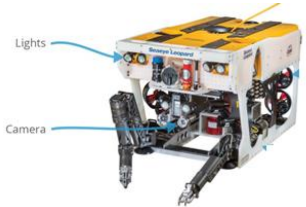
Şekil 3. ROV Uzaktan Kumandalı Sualtı Aracı ( https://bluerobotics.com ). Figure 3. ROV Remote Controlled Underwater Vehicle ( https://bluerobotics.com ).
