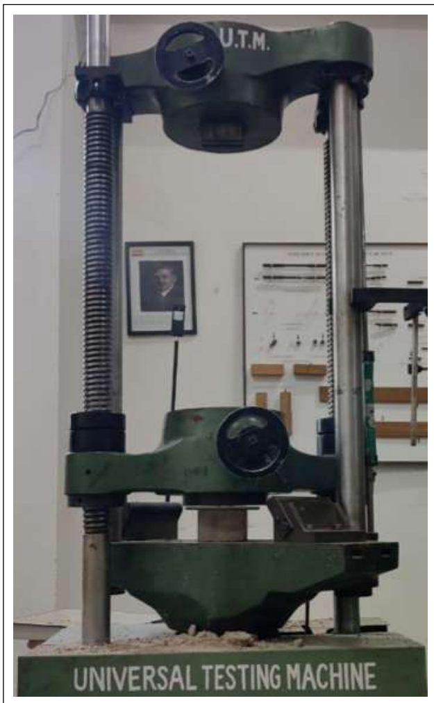
Figure 4. Universal testing machine.
