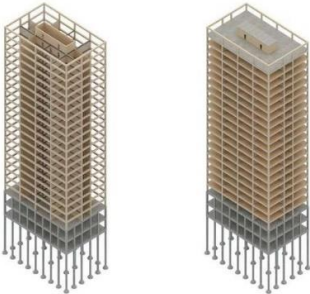
Şekil 6. Prefabrike Ahşap Karkas Sistem (The Future Academic Plaform, 2023)
