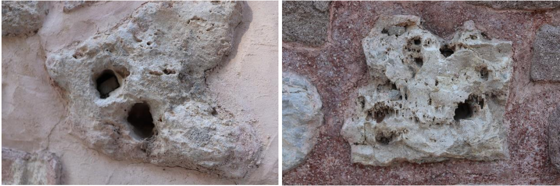
Figure 10. Macropores that occur in the formation of the stone appear as holes on the surface
