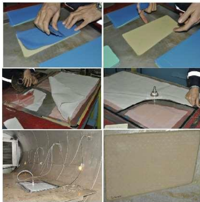
Figure 3. Composite Test Panel Manufacturing
