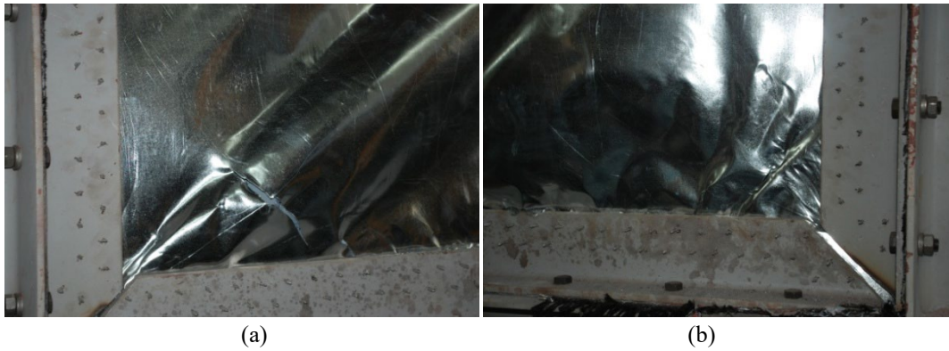
Figure 9. CLB specimen ( +10\delta y ) step (a) 80 mm tearing from the lower left edge (b) no tearing at the lower right edge
