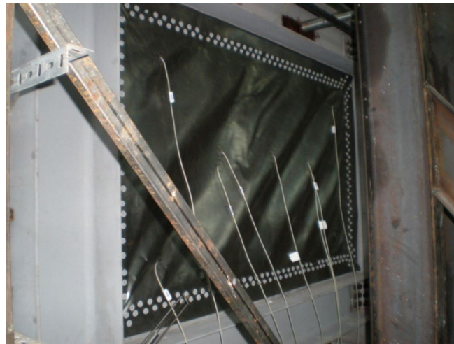
Figure 10. General view of the TL specimen at the +5\delta y displacement step (30.13 mm)
