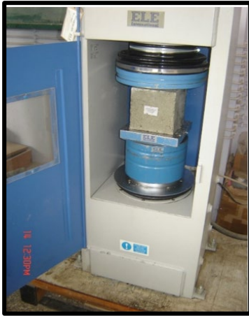
Figure 4. Concrete compressive strength test.
