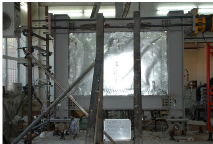
Figure 2. CLB specimen double-layer steel plate shear wall with CFRP (+2/3*δy; 4.02 mm)
