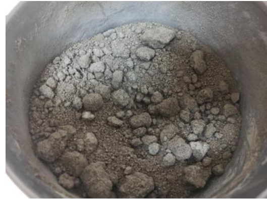
Figure 1. Solidification of the mixture with a preheating temperature of 75°C during the mixing process
