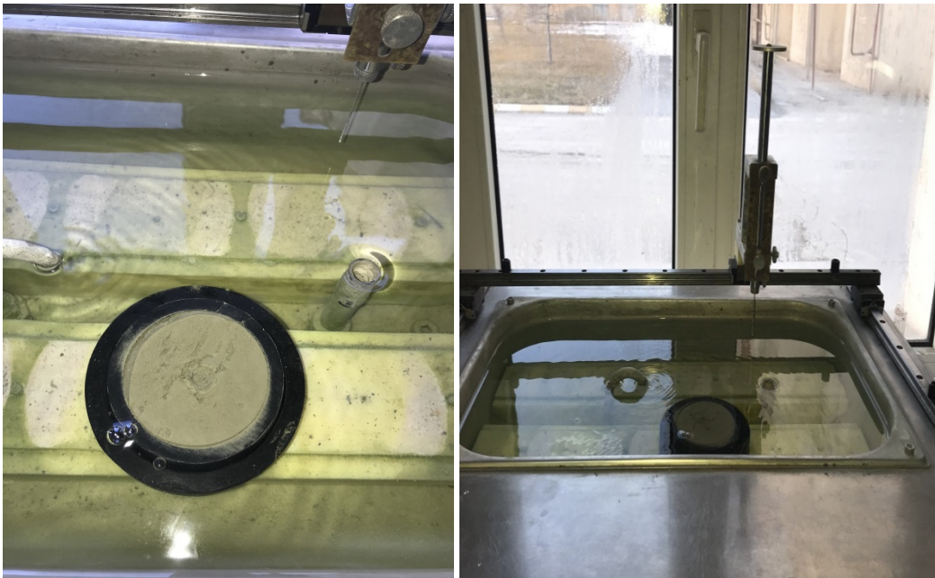
Figure 4 Setting time experiment (Using Vicat Tool).
