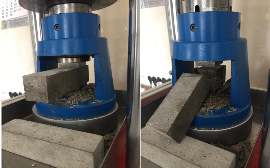
Figure 5. Compressive strength experiment.
