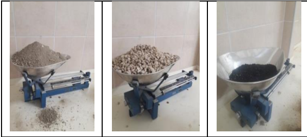
Şekil 3. İnce, kaba ve lastik agrega Figure 3. Fine, coarse and rubber aggregate
