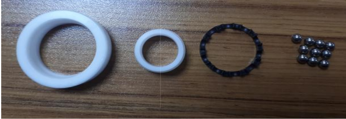
Figure 1. The distributed view of polymer hybrid deep groove ball bearing
