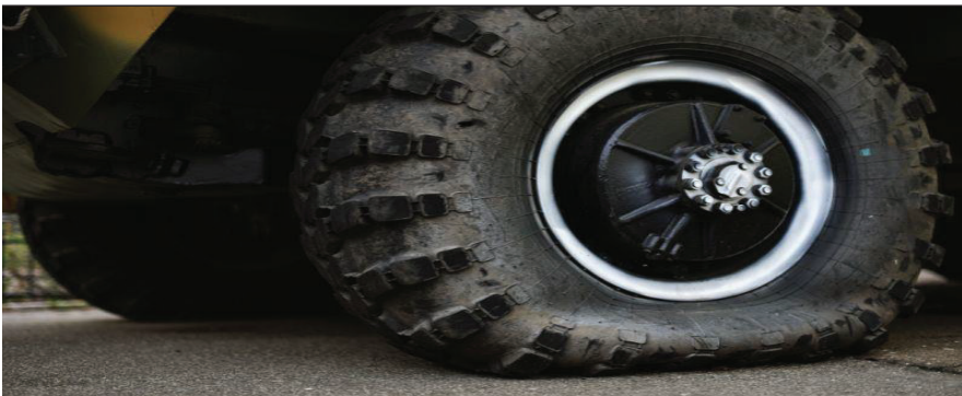
Figure 3. Run Flat Tire in the Event of Loss of Pressure
