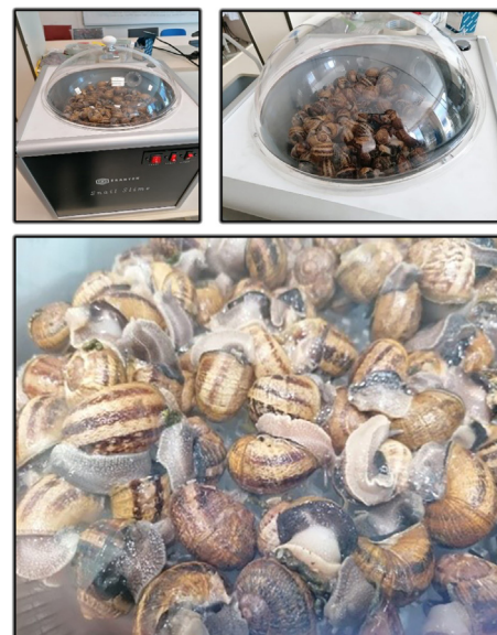
Figure 2. Treatment of snails with cold steam containing ozone and essential oil in a specially designed device
