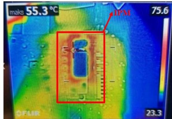
Fig 16. IPM temperature graph at tested switching
