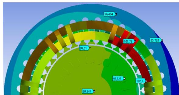
Fig. 11. Side section temperature dispersion
