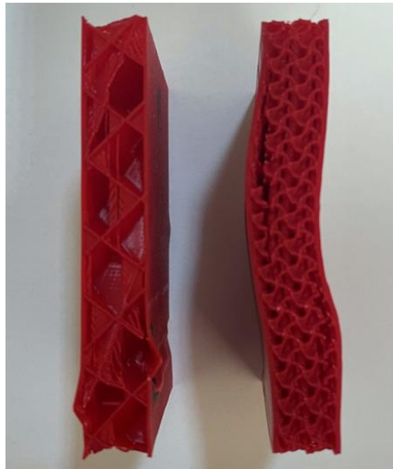
Figure 3. Unacceptable and acceptable types of damages
