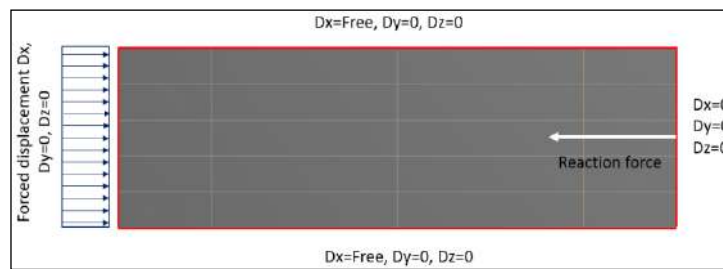
Figure 7. Forced displacement application and boundary conditions
