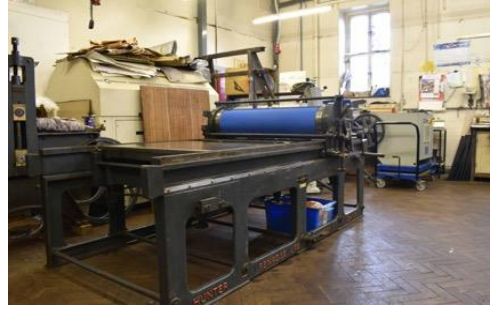
Görsel 1. Northamptonshire, 2023, Hunter-Penrose litografi presi / Hunter-Penrose lithography press.
