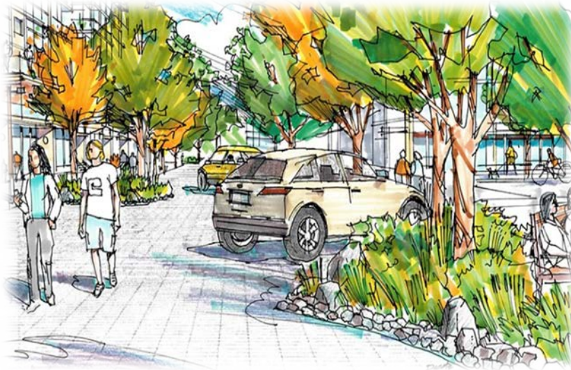
Figure 3. Source (URL-2). The illustration shows an imagined example of Woonerf. It shows parking places, planting trees as obstacles, and how pedestrians use the whole street.
