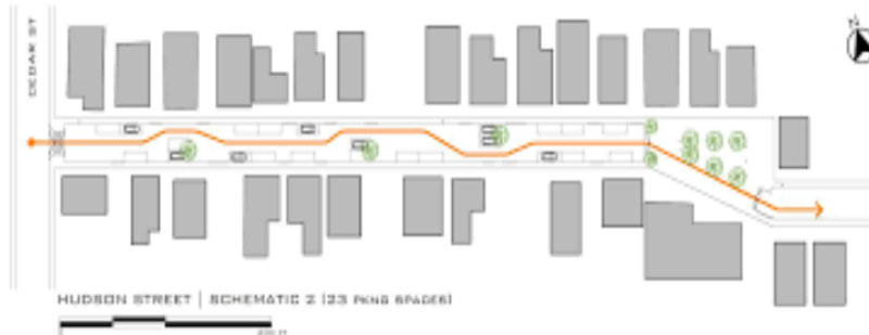
Figure 4. A sketch shows how obstacles and parking places can be distributed on Woonerf Street. Source (Collarte, 2012).
