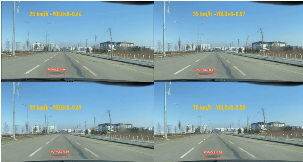
Figure 7. Detection performance of YOLOv8 on the same road and pothole at 25-35-50-70 km/h
