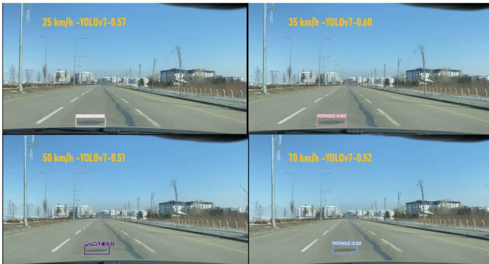
Figure 6. Detection performance of YOLOv7 on the same road and pothole at 25-35-50-70 km/h
