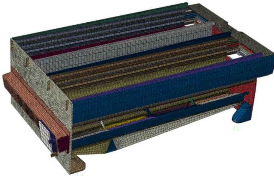
**Figure 10.** Finite element model of purifier machine
