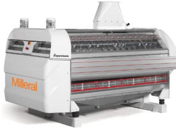
**Figure 2.** Semolina purifier machine
