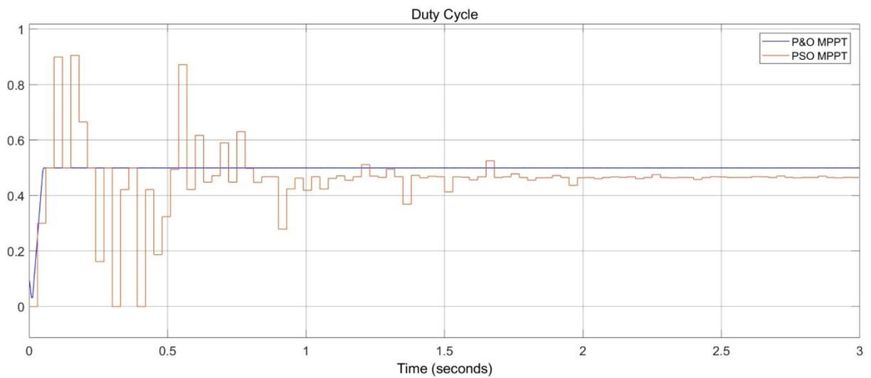
**Figure 10.** Duty cycle change for the P&O and PSO
