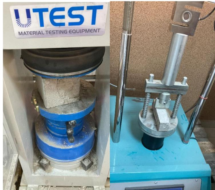
Figure 2. Compression and flexural test
