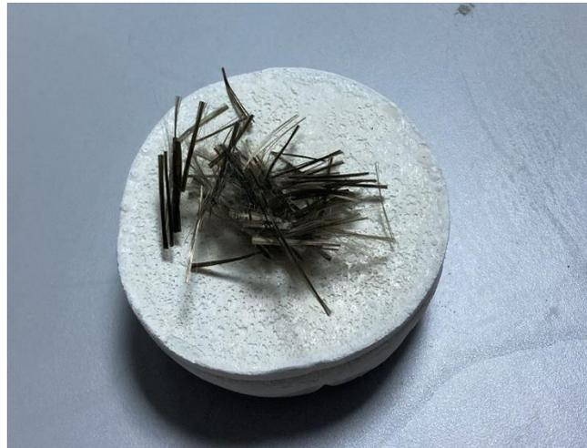
**Figure 1.** Basalt fibers
