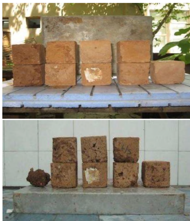
Figure 7. Water absorption test.
