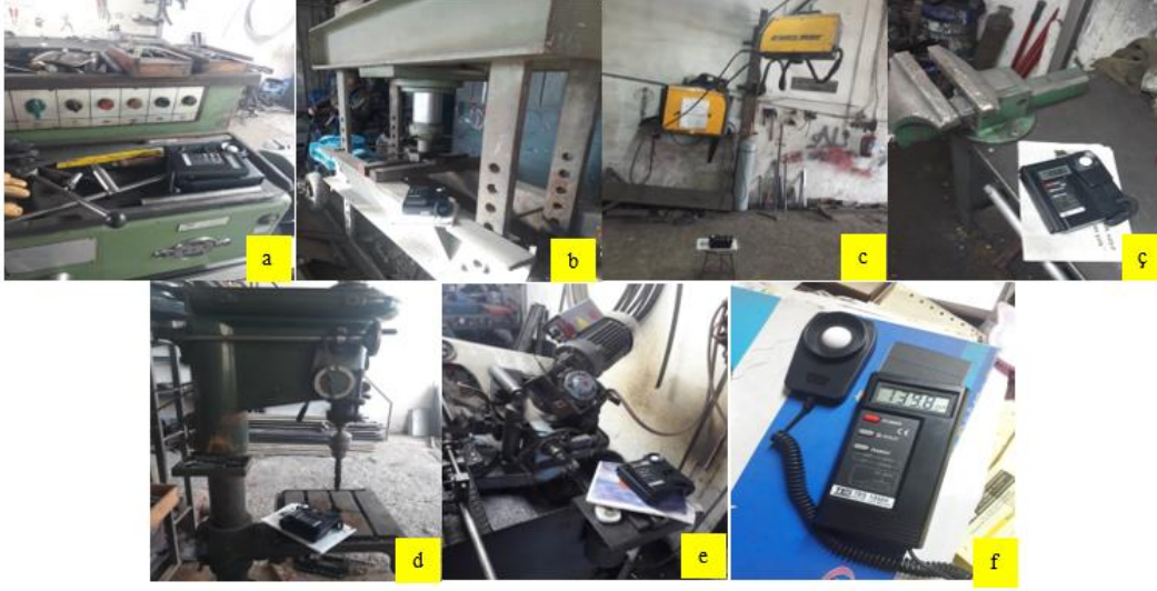
Figure 2. Places where lighting measurements are made within the company (a: Lathe bench b: Press machine c: Gas metal arc welding ç: Vice d: Column drill e: Saw cutting f: Administrative office)
