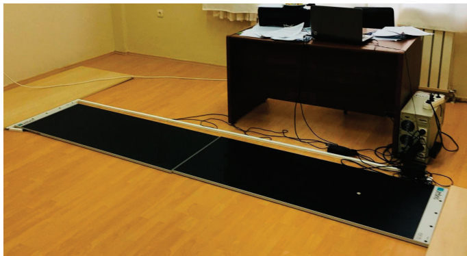
Figure 2. The force platform Zebris©, FDM System Type FDM 1,5 and WinFDM computer program.
