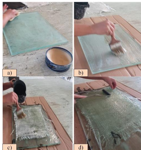
Figure 2. (a) Surface application of wax (b) Resin application (c) Resin application between fiber layers (d) Using a roller to remove excess resin
