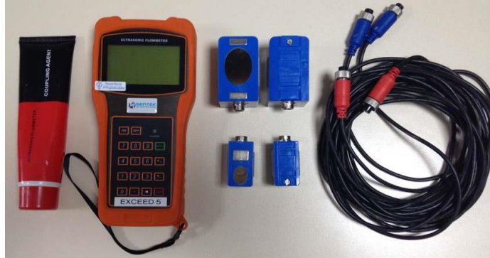
Şekil 2. TFM1100-P modeli portatif ultrasonik debimetre (TFM1100-P model portable ultrasonic flowmeter)
