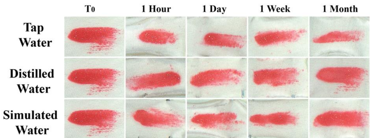
Figure 16. Stability test of lip gloss on fabric.
