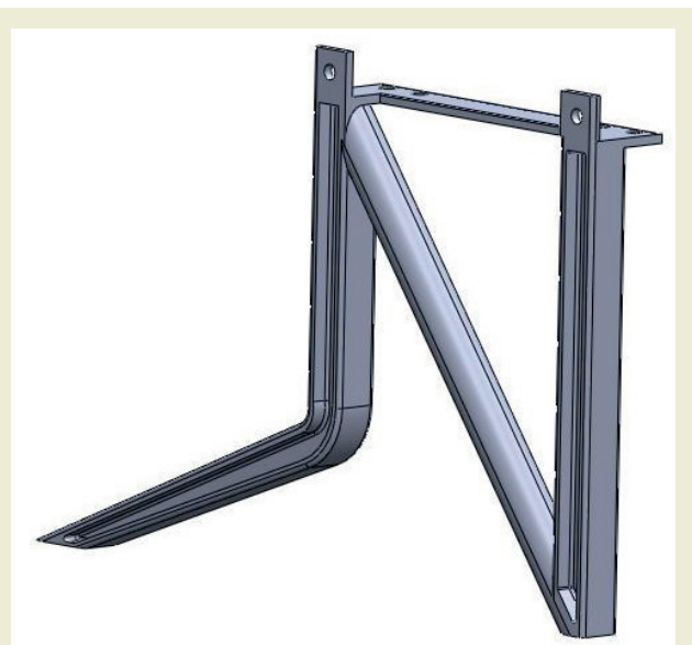
Figure 33. Improved design via topological optimization for simulation 1.
