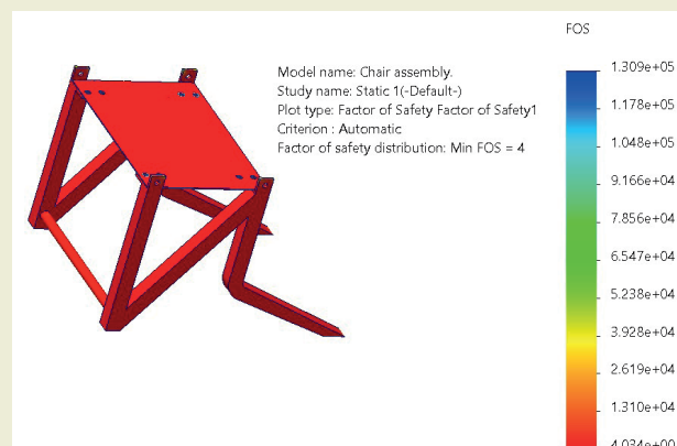
Figure 16. Failure Criteria (factor of safety) computed In SOLIDWORKS for simulation 1
