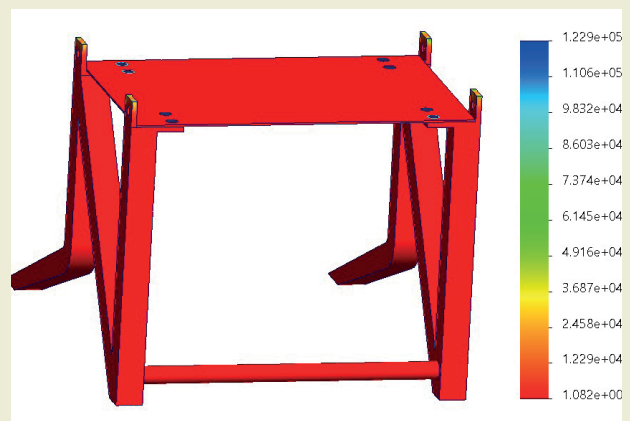
Figure 29. Failure Criteria (factor of safety) computed In SOLIDWORKS for simulation 4.
