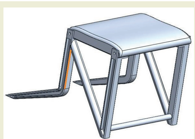
Figure 34. Fully Assembled Optimized Seat Frame (for simulation 1-AL7075-T6(SN)).
