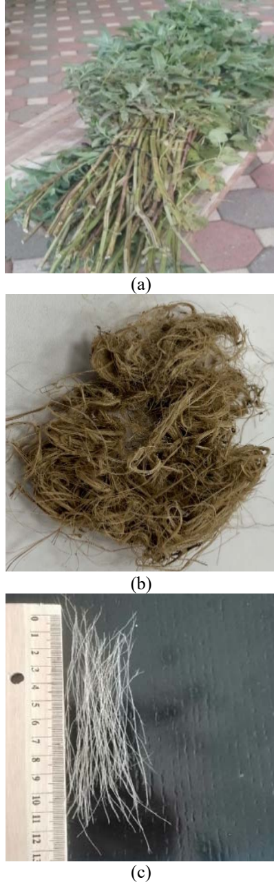
Figure 1. The digital images of (a) MPL plant, (b) obtained MPL stem fibers (c) combed MPL samples
