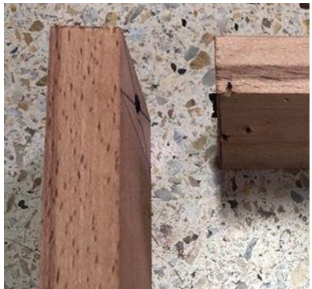
Figure 7. Resin Dowel Joint Failure
