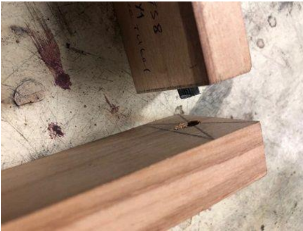
Figure 8. Plastic Dowel Failure
