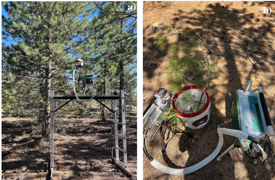
Figure 2. Measurement of gas exchange parameters by a) in-situ method and b) in-vitro method
