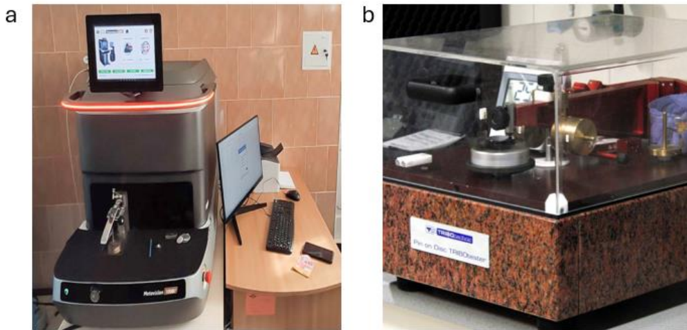
Fig. 3. (a) optical emission spectrometer; (b) wear test device.
