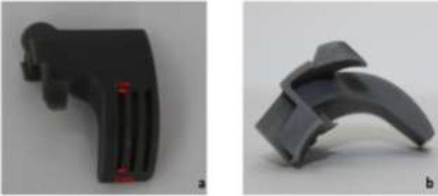
**Figure 4.** 3D printed suction-insert for compact three-roving yarn a) front view b) side view
