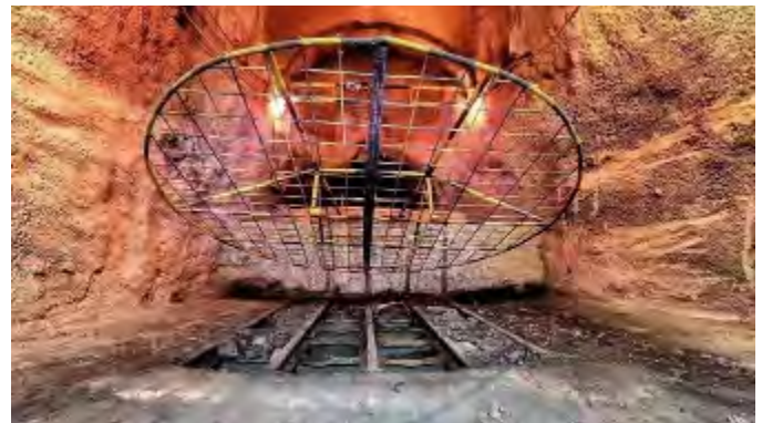
Fig.2 Opened ore pass cover
