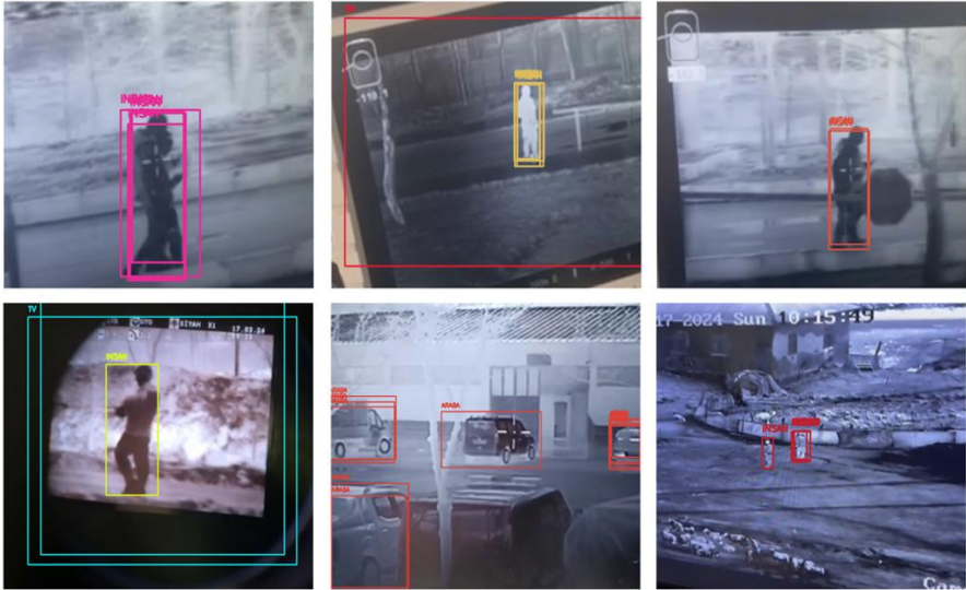
Figure-9. Thermal images experimented via YOLO v3.
