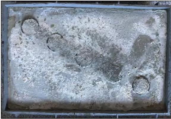
Figure 4- Casted concrete and impregnated cylindrical core samplers.
