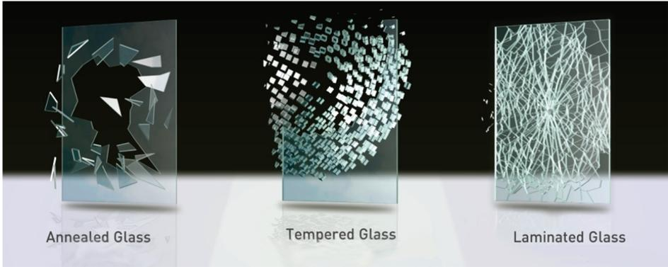
Fig. 1 - Typical fracture shapes of glass types [1]
