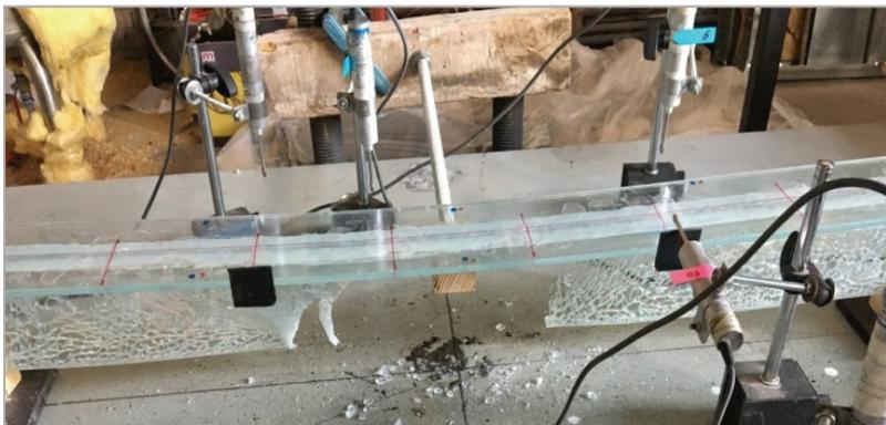
Fig. 17 - Tempered glass T-beam exposed to its ultimate loading
