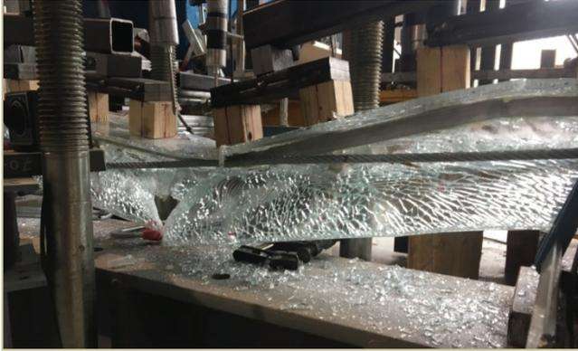
Fig. 21 - Post-tensioned tempered glass T-beam after fracture.
